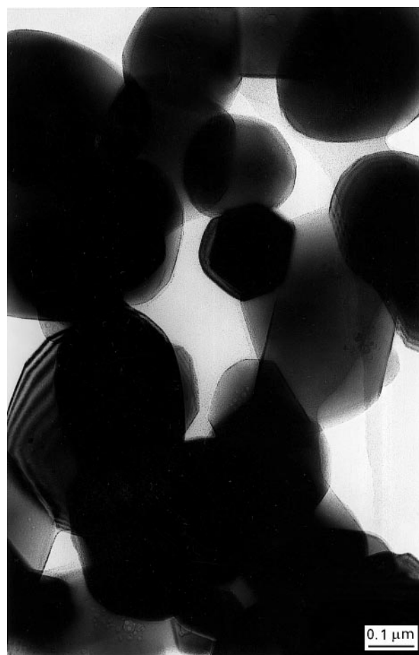
Figure 14 TEM micrograph of \text{TiO}_2 coated with carbon reaction product at 1500^\circ\text{C} for 2 h in flowing argon.
